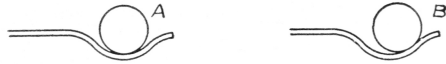
Figure 197—A, correctly shaped spring. B, incorrectly shaped spring which may cause the split hand to jump when released.
